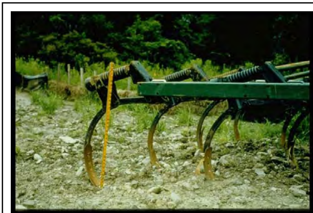
Fig. 6. A light duty chisel implement, not adequate for either the deep ripping or decompaction (deep subsoiling) phase.
